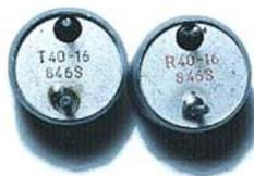
Gambar 14. Ultrasonic transmitter (T40-16) dan receiver (R40-16) (tampak belakang)
